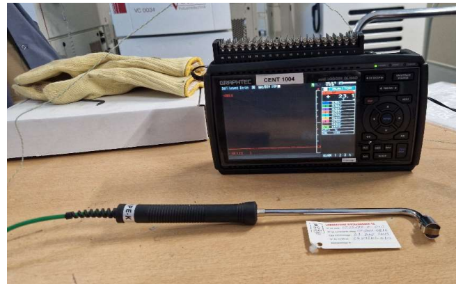
Thermal Probe (measuring capability up to 1000°C)
