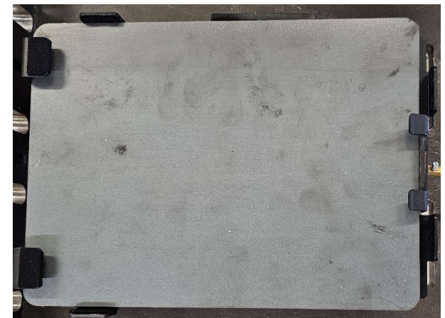
Steel Plate (250 x 180 x 5 mm) (to simulate the overheating iPad for the test) Qty 3
