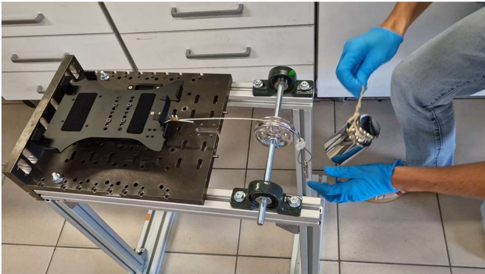
Test of cradle opening mechanism “before” thermal runaway simulation, with 2.0 Kg → ~ 70% opening
