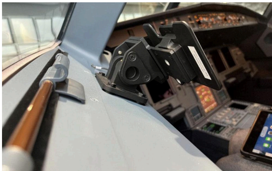
(fig.10) Example of a cockpit mount for tablets recommended as an option on A320 family aircraft
